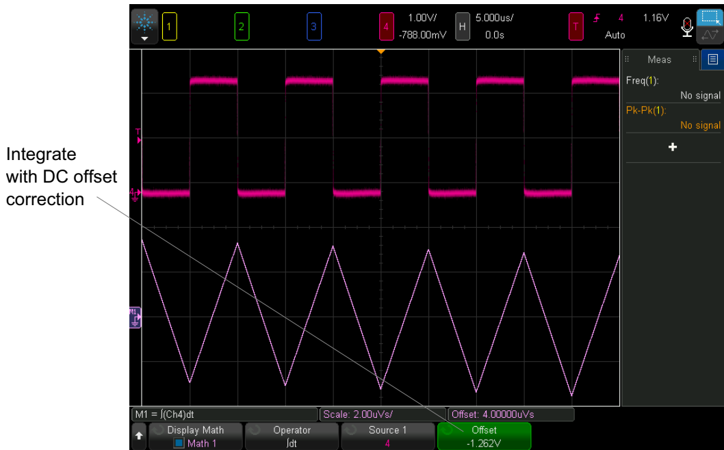
Figure 9 Integrate With Signal Offset
