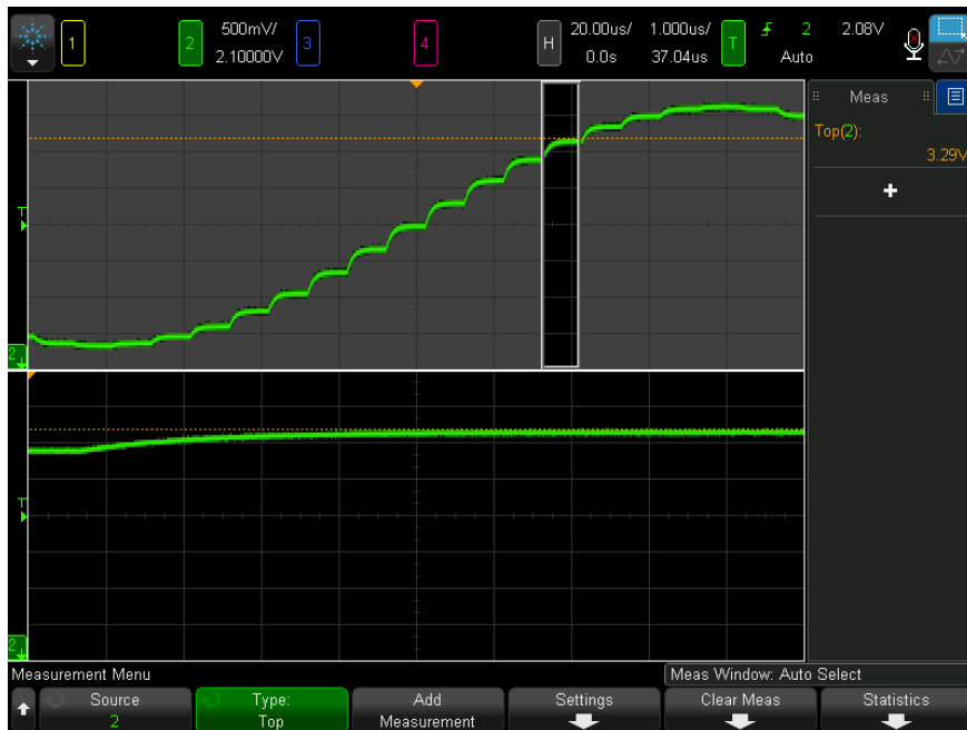
Figure 47 Isolating area for Top measurement
