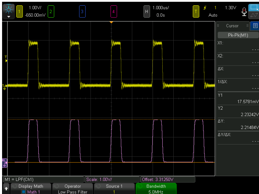
Figure 16 Example of Low Pass Filter
